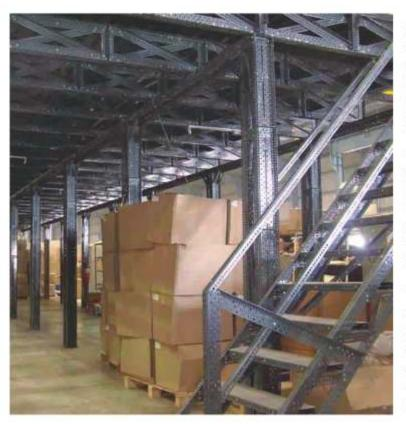
**SPANCO** Mezzanine Floors are fabricated, supplied and installed as per the clients demands. These floors can be made on top of heavy duty pallet racks, or just with heavy duty pillars, or with Slotted Angles.
