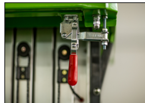
Fixture for Platform Guardrail
