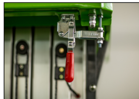
Fixture for Platform Guardrail
