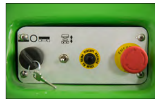
Ground Control Panel
