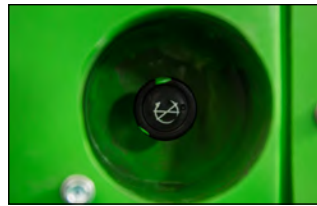
Emergency Descend Valve
