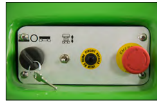
Ground Control Panel
