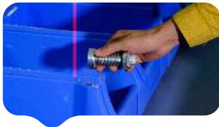
LASER POINTER FOR MATERIAL LOCATION
