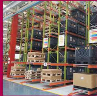
Very Narrow Aisle Racking
