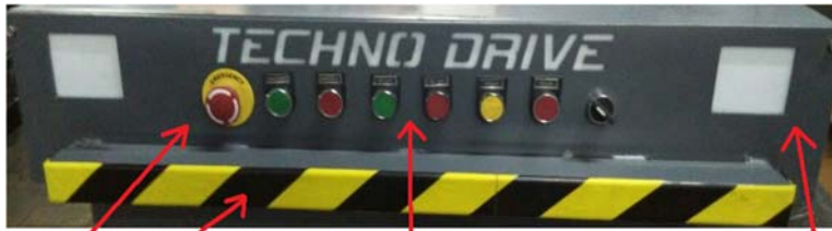
EMERGENCY BUTTON SAFETY BAR
