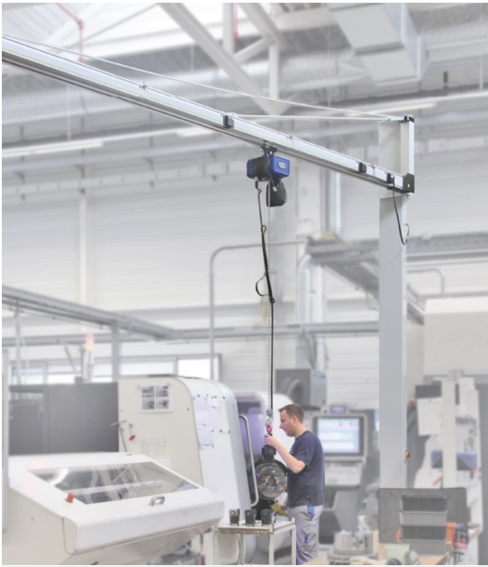
Jib Crane and Hoist for loading and unloading CNC machine
