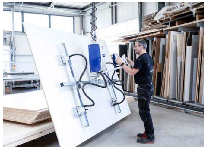
Pneumatic vacuum lifting device VacuMaster Wood, 90° swiveling, for transporting wooden boards from the storage to the saw
