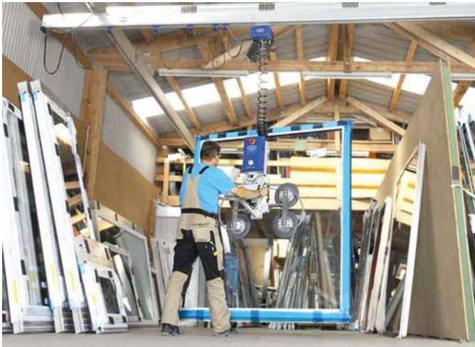
Vacuum lifting device VacuMaster Window Comfort for handling windows, glass panes and glass components
