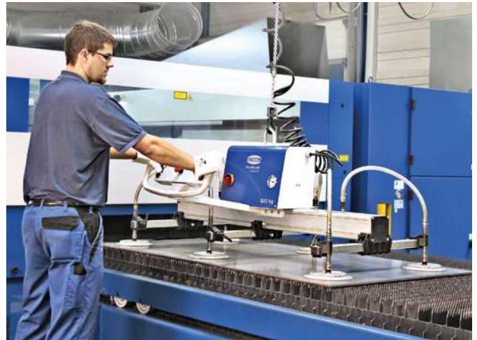
Vacuum lifting device VacuMaster Comfort for loading and unloading a laser cutting machine
