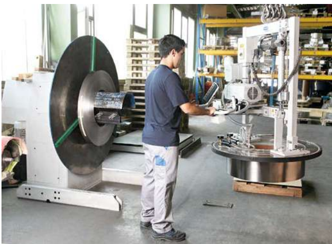
Vacuum lifting device VacuMaster Coil with 90° swivel angle for handling coils
