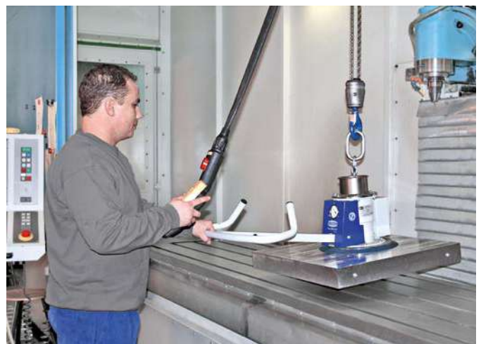
Vacuum lifting device VacuMaster Eco for energy-independent handling metal parts
