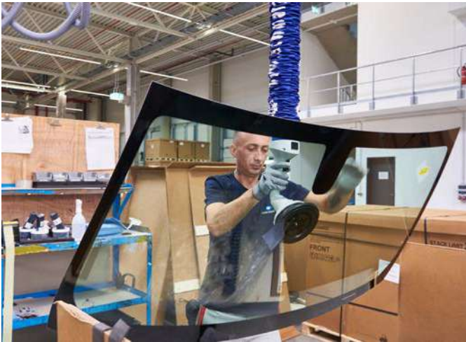
Vacuum tube lifter JumboFlex for handling windshields
